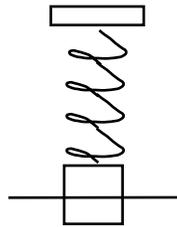
Now we have a spring attached to the ceiling, and a block (with mass  $m$ ) attached to the bottom end. The spring is (for the moment) sitting at equilibrium. Let's think of this equilibrium location as  $y = 0$ . We're going to pull the block downward (we will think of that as a positive  $y$ -value), and then release it.
