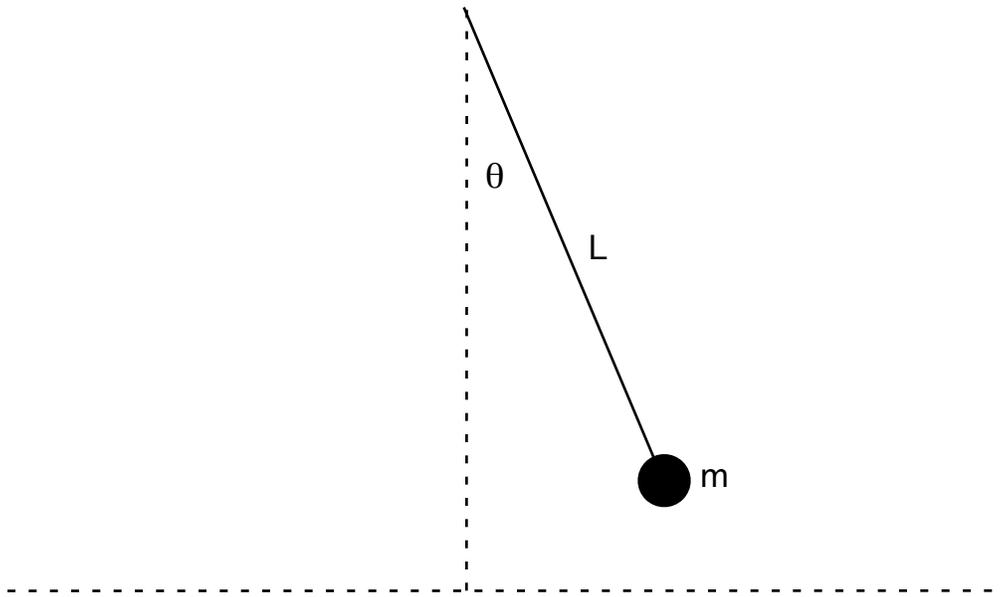
A pendulum has a bob on the end. It is set into motion by being pulled to the right (or being pushed to the left) a certain angle and then being released. The resulting angle is sinusoidal (i.e. has a graph like a sine or cosine wave).
